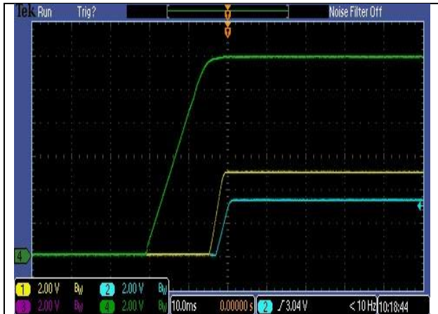
Extended Name = 12V 5V 3.3V Power Sequence - DSO Image Capture - 115/60V Light Load (20%) Var Name = Power OK Rise Time
