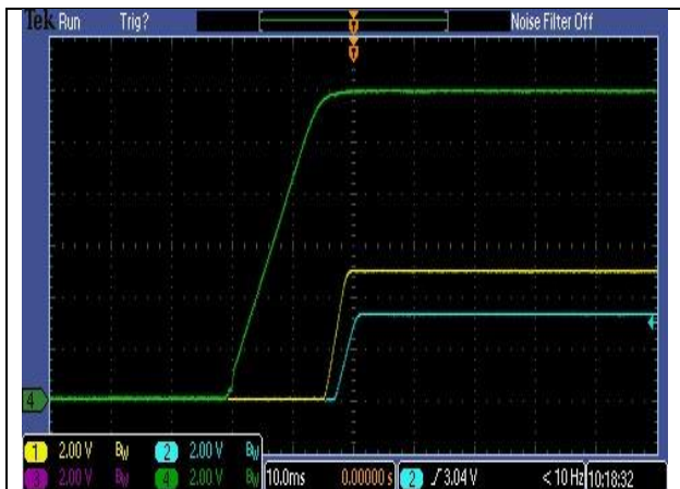
Extended Name = 12V 5V 3.3V Power Sequence - DSO Image Capture - 115/60V Typical Load (50%) Var Name = Power OK Rise Time
