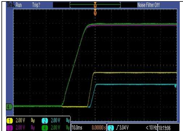
Extended Name = 12V 5V 3.3V Power Sequence - DSO Image Capture - 115/60V Full Load (100%) Var Name = Power OK Rise Time
