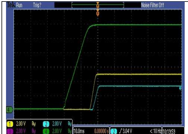
Extended Name = 12V 5V 3.3V Power Sequence - DSO Image Capture - 230/50V Typical Load (50%) Var Name = Power OK Rise Time
