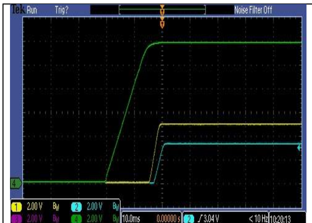
Extended Name = 12V 5V 3.3V Power Sequence - DSO Image Capture - 230/50V Light Load (20%) Var Name = Power OK Rise Time
