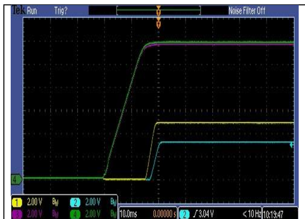
Extended Name = 12V 5V 3.3V Power Sequence - DSO Image Capture - 230/50V Full Load (100%) Var Name = Power OK Rise Time
